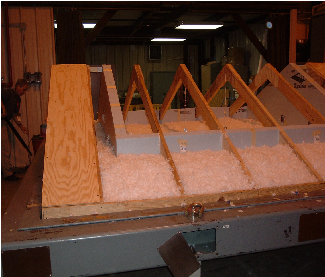
Figure 1. Photograph of Attic Test Module without Roof Sheathing
